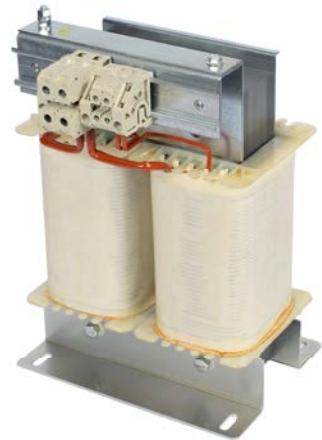
Transformers for powering group-2 medical premises, through galvanic separation between the power supply network and the user load. The insulation between the primary and secondary windings is double and reinforced, made with an UL CSA-certified insulating system.
