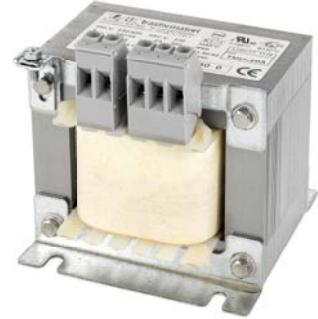
Approved transformers for safety circuits. The insulation between the primary and secondary winding is double and created with the UL CSA certified insulation system. Primary with adjustment sockets.
