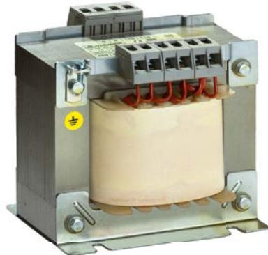
Manufactured in compliance with CEI EN60601-1 for incorporation in electromedical devices. The distinctive features of this transformer are the overheating protection of the basic insulation, the supplementary insulation, and the reinforced insulation in the event of short circuit or overload of each output winding.
