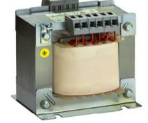
Manufactured in compliance with CEI EN60601-1 for incorporation in electromedical devices. The distinctive features of this transformer are the overheating protection of the basic insulation, the supplementary insulation, and the reinforced insulation in the event of short circuit or overload of each output winding.
